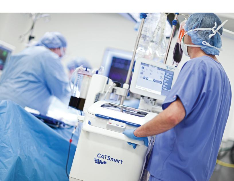
At the heart of CATSmart is our proprietary continuous-flow technology. Unlike bowl-based systems, its one-size-fits-all kit multi-tasks all process steps. Coupled with situation-specific wash programs, an Auto-Start function, and a PRC pump sensor, you can set up fast and be certain PRC is available when your patient needs it.
